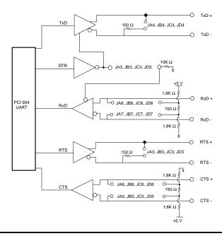
Figure 8: RS-422/485 partial schematic for Rear I/O Opto
